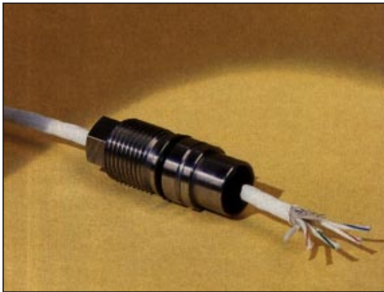
Top seal. Designed for the new Propfan jet engine, this seal has a stainless steel housing that protects the shielded Teflon wires at pressures of up to 100 psi of nitrogen, temperatures of -65^{\circ} to 390^{\circ} F, severe vibration, and a 50-lb pull test load on individual wires.
